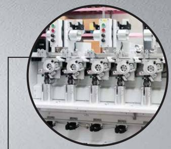
The **ROTOSOFT** machine has been designed and realized for high versatility functions in order to fulfil the various demands of the yarn fashion-market. Each section is composed of eight positions with possibility of different yarn style every 2 – 4 or 8 spindles.
