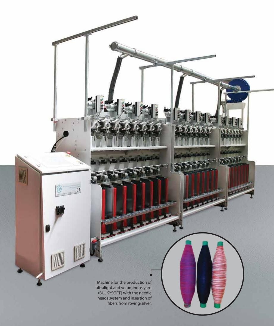
By some simple adjustments, which precision is granted by the electronic control system the ROTOSOFT can be easily set up to produce yarns that repeat exactly the quality and characteristics needed by the garment design both in hand knitting and machine knitting. The possibility of using different yarn types for the tubular net and different type of fibers for the inserted effect make the ROTOSOFT a flexible machine that fully meets all the production requirements.
