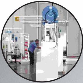
The number of spindles suggested to assign to an operator depends on the yarn count produced. Indicatively for count Nm 2 can be up to 120 spindles, with a production of approximately 330 Kg of yarn in the 8 hours, which are becoming the approximately 1000 Kgs in the 24 hours.
